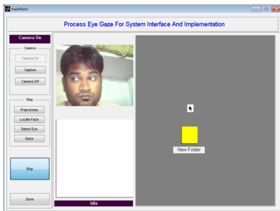
Fig.4. Movement of Cursor in upward direction and camera take next image snap for next movement (left side)
